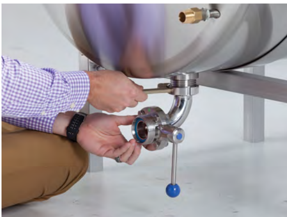
FIGURE 16: PIERCING VALVE REMOVAL
