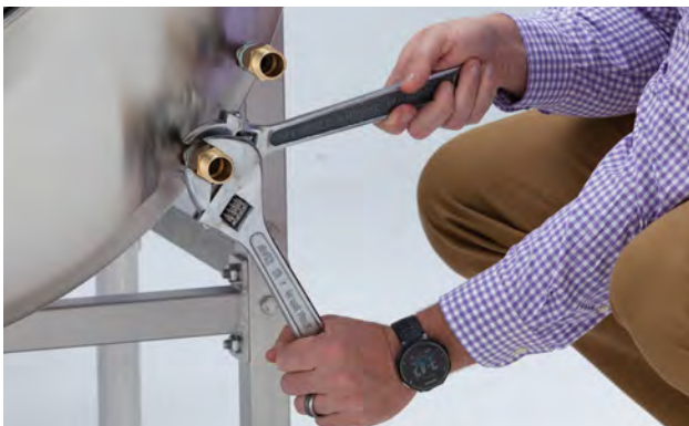
FIGURE 12: WATER COOLING CONNECTION
