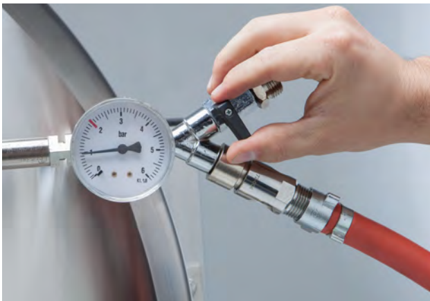
FIGURE 18: ADJUSTING TANK PRESSURE
