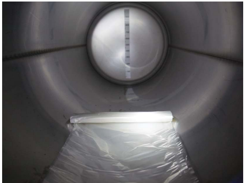
Inliner placed and ready to receive fresh beer.
